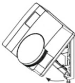
Once the batteries are fitted, re-fit the thermostat to the wall plate by engaging with the lugs at the top of the wall plate and push the thermostat into position. Locate it over the captive screws at the base of the wall plate and tighten so that the thermostat is locked into position.
