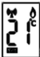
The aerial symbol complete with radio wave symbols in the display of the thermostat indicates that it is communicating satisfactorily with the CentaurPlus C17-ZW.
