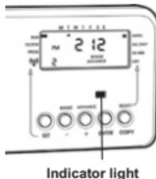
When the timeswitch is 'On' (shown by the red indicator light) the thermostat will be operational and will provide very accurate control of the room temperature.
